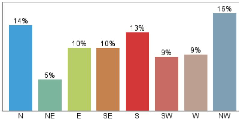
The fraction of time spent with the wind blowing from the various directions over the entire year. Values do not sum to 100% because the wind direction is undefined when the wind speed is zero.
